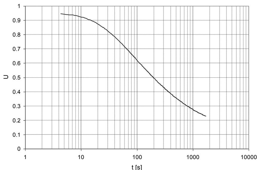
Fig. 10. Normalized excess pore water pressure (Bałachowski, 2006b)
