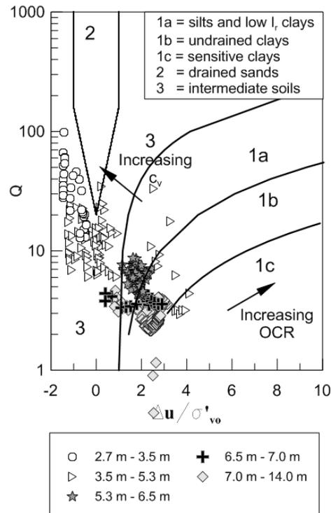
Fig. 8. Foynes CPTU data plotted on chart of Schneider et al. (2008).
