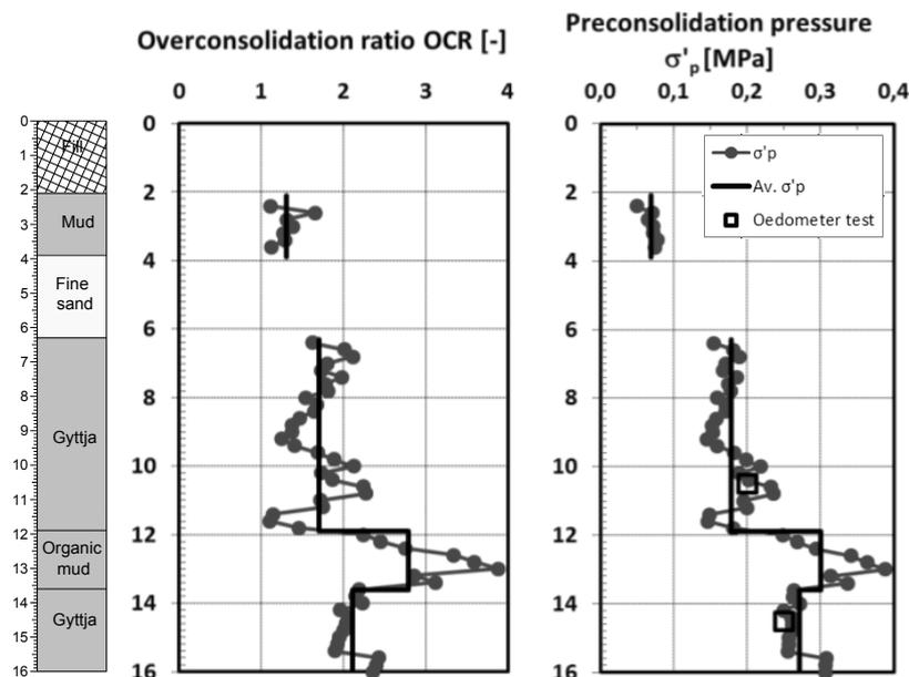
Fig. 4 – Profiles of the overconsolidation ratio OCR and the preconsolidation pressure  $\sigma'_p$  from the SDMT test and values obtained from the oedometer test for the subsoil of the Plocka Station
