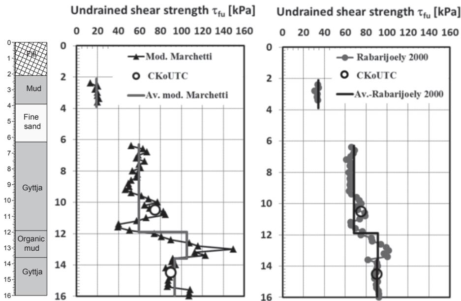
Fig. 5 – Undrained shear strength from the SDMT test and the CK<sub>0</sub>U triaxial test for the subsoil of the Plocka Station
