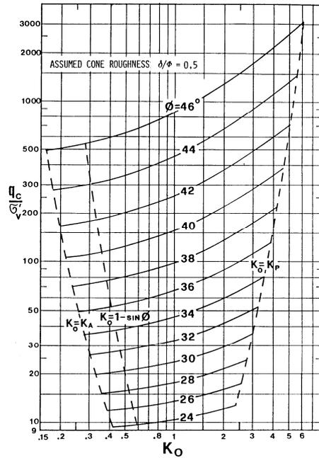
Fig. 4.2 Interrelationship  $q_c$ - $\phi$ - $K_o$  by Durgunoglu and Mitchell (1975). Converted in graphical format by Marchetti 1985.
