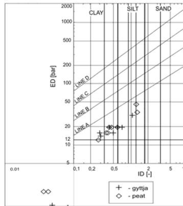
Fig. 4. Position of tested organic soils in the classification diagram by Marchetti and Craps (1981)
