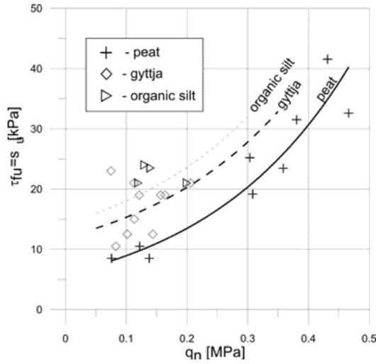
Fig. 10. Differences in correlation trends between maximal shear stress  $\tau_{fU}$  from VT and net cone resistance  $q_n$  for different soil types
