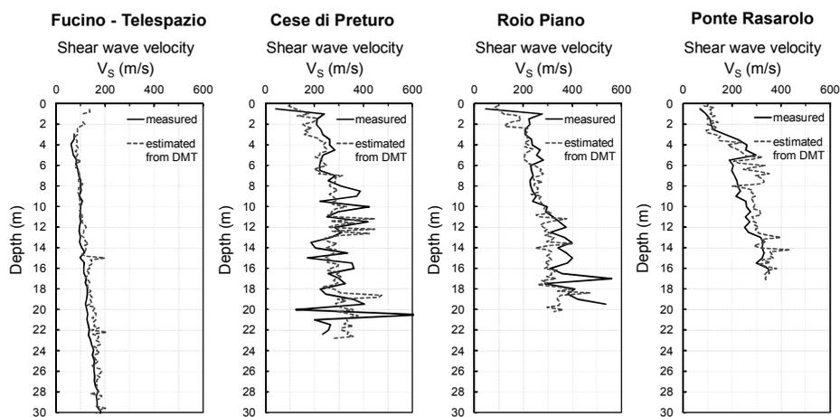
Fig. 8. Comparison of profiles of  $V_S$  measured by SDMT and estimated from DMT data at four silty-clayey sites in Abruzzo, Italy
