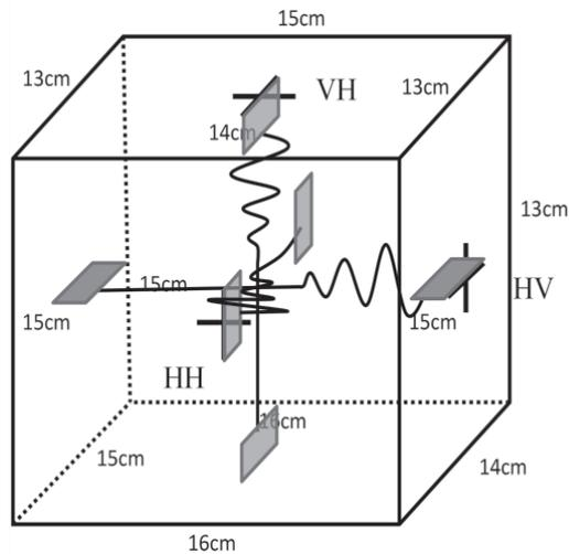
Fig. 10 Setting the bender element for measurement of anisotropy of  $G$ Tab. 1 Measured  $G$  for different direction
