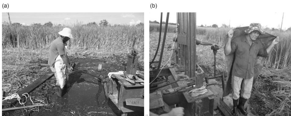
Fig. 11. (a) Beginning of a seismic test; (b) Protection against water splashing when the weight of a person is required to keep the hammer stable.
