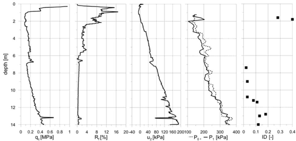
Fig. 3. Typical CPTU and DMT characteristics for Stargard Szczeciński test site.
