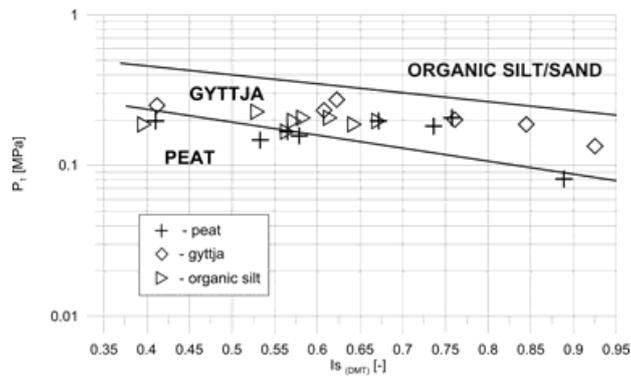
Fig. 5. Position of tested soils in the classification diagram by Rabarijoely (2013)
