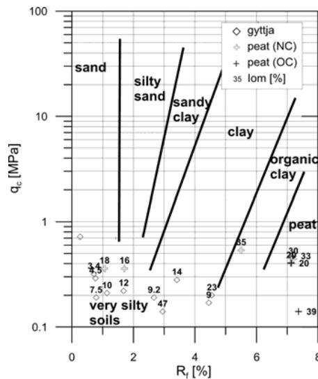
Fig. 8. Location of investigated soils in the classification diagram by Schmertmann (1969), numbers denote contents of organic fractions  $I_{om}$ .
