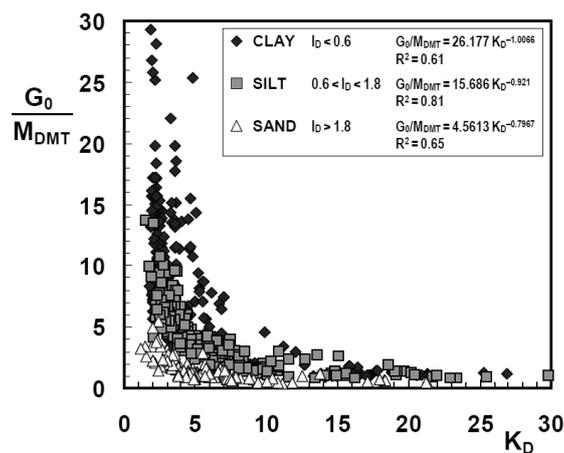
Fig. 7. Ratio  $G_0/M_{DMT}$  vs.  $K_D$  (OCR) for various soil types (Monaco et al. 2009)
