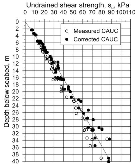
Fig. 8. Measured and corrected undrained shear strength from CAUC triaxial tests
