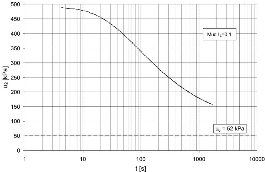
Fig. 9. Typical dissipation curve in NC soils under the central part of the dike (Bałachowski, 2006b)
