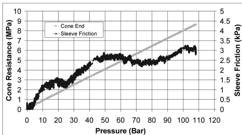
Fig. 2. Calibration of Beta factor (Sleeve vs chamber pressure )
