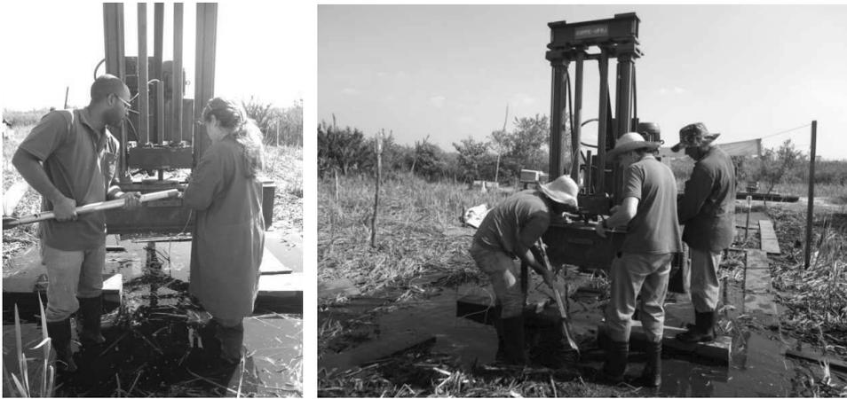
Fig. 10. Handling the seismic dilatometer in the beginning of the test.
