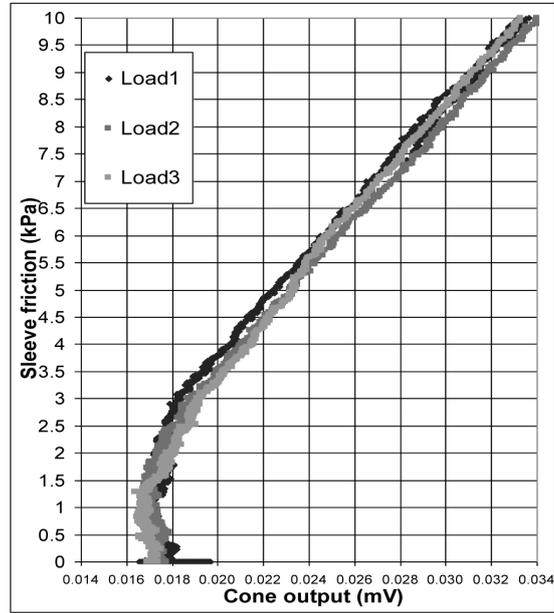
Fig. 8. Sleeve measurements on classic cone design
