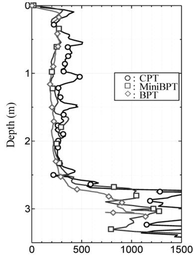
Fig. 4. Comparison of CPT and BPT
