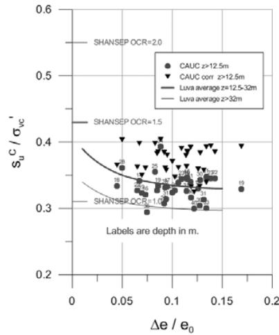
Fig. 11. Comparison of triaxial compression strength determination,  $z > 12.5$  m
