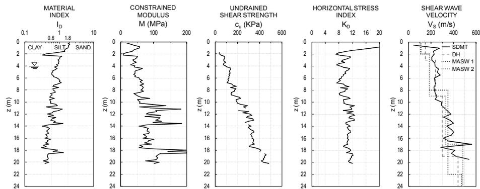
Fig. 5. SDMT results at the site of Roio Piano (C.A.S.E. Project), L'Aquila. *On the right*: Comparison of profiles of  $V_s$  from SDMT, Down-Hole (Polo Geologico) and MASW (Politecnico di Torino). DH and MASW data from MS–AQ Working Group (2010); see also Santucci de Magistris et al. (2013).
