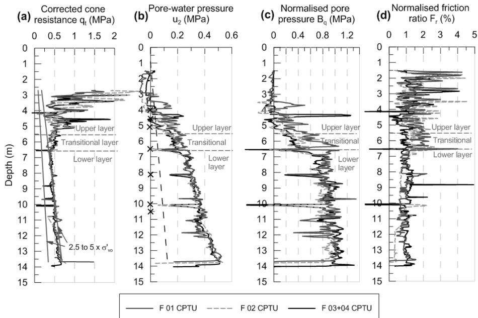
Fig. 4. Results of CPTU tests at Foynes
