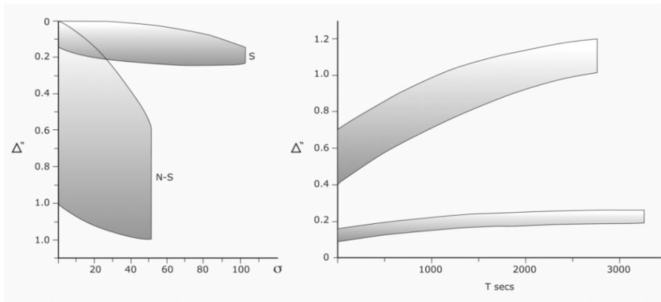
Fig. 6. Deflection against stress compared, (left), for stabilised (S) and non-stabilised (N-S) And corresponding applied stress histories, (right)
