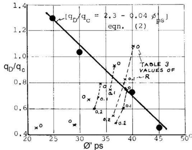
Fig. 8.1 Predicted  $q_d/q_c$  from D&M theory (Schmertmann 1982)
