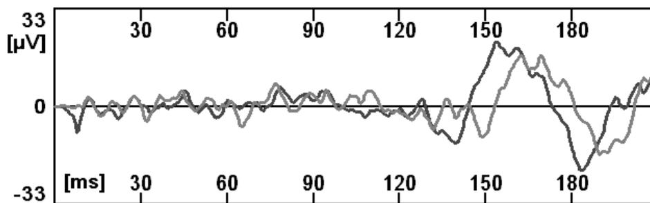
Fig. 13. Shear wave in SDMT02/01, 6.0 m depth,  $v_s = 56$  m/s.
