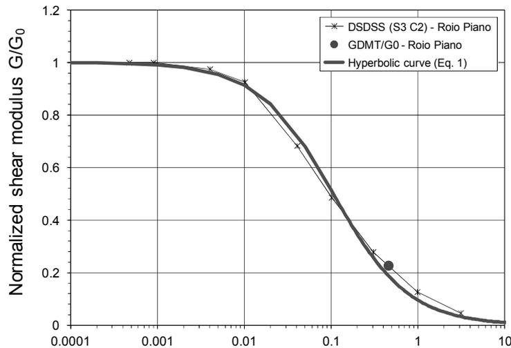
Fig. 10. Roio Piano, L'Aquila – Comparison between  $G/G_0 - \gamma$  decay curves estimated from SDMT by Eq. (1) and „measured” in the laboratory (DSDSS: double sample direct simple shear tests, University of Roma La Sapienza, Santucci de Magistris et al. 2013) (Amoroso et al. 2014)
