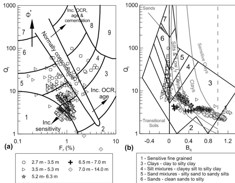
Fig. 7. Foynes CPTU data plotted on Robertson (1990) soil behaviour charts (a)  $Q_t$  versus  $F_r$  and (b)  $Q_t$  versus  $B_q$ .
