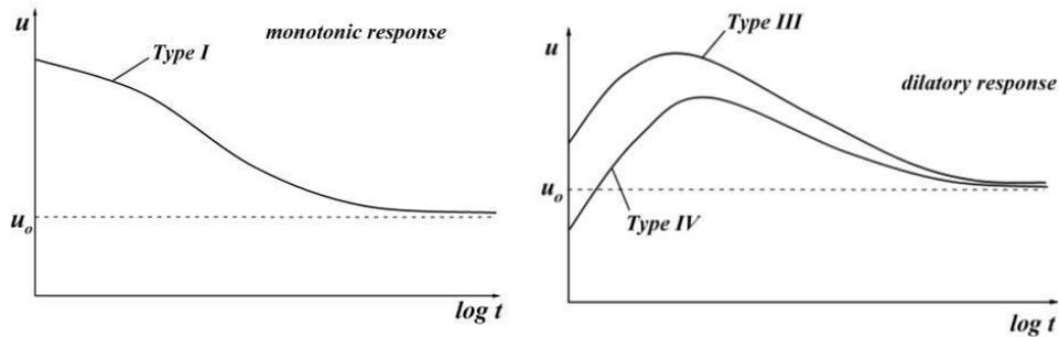
Fig. 8. Typical dissipation curves in normally consolidated and overconsolidated soils (after Sully et al. 1999)
