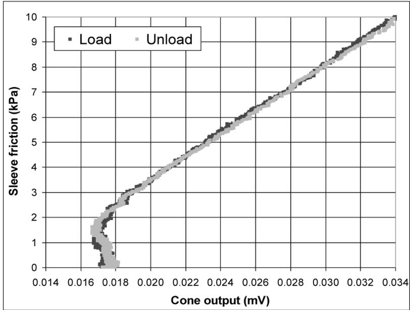
Fig. 10. Load – Unload on classic cone design
