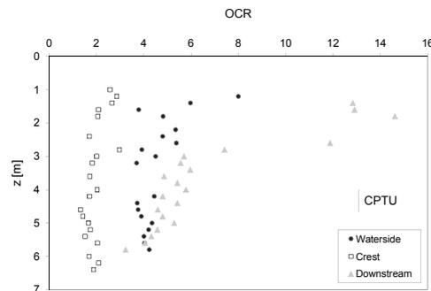
Fig. 3. Overconsolidation ratio of the dike subsoil from CPTU
