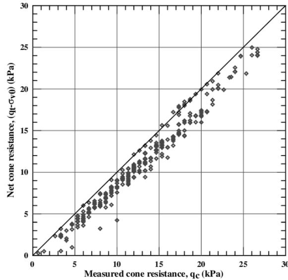
Fig.12. Comparison of  $q_c$  and  $q_{net}$
