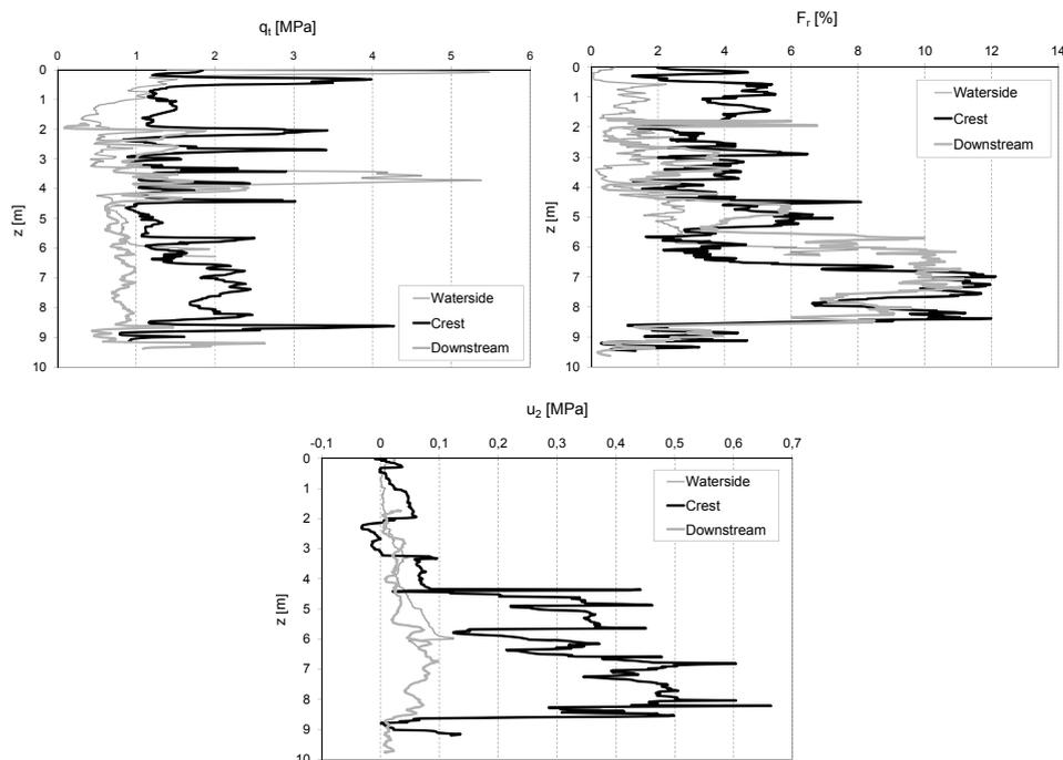
Fig. 2. CPTU tests in a typical cross section of the dike
