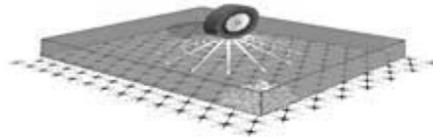
Fig. 2. Radial distribution of load from traffic (EOTA 2012)
