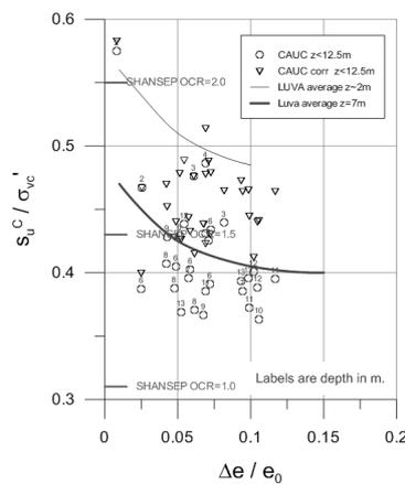
Fig. 10. Comparison of triaxial compression strength determination,  $z < 12.5$  m
