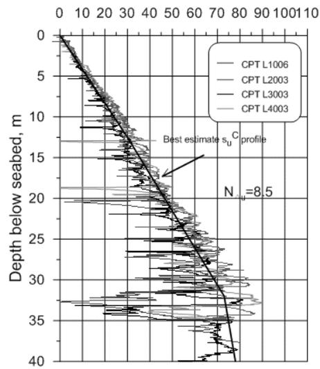
Fig. 14. Undrained shear strength from CPTU,  $N_{\Delta u}$
