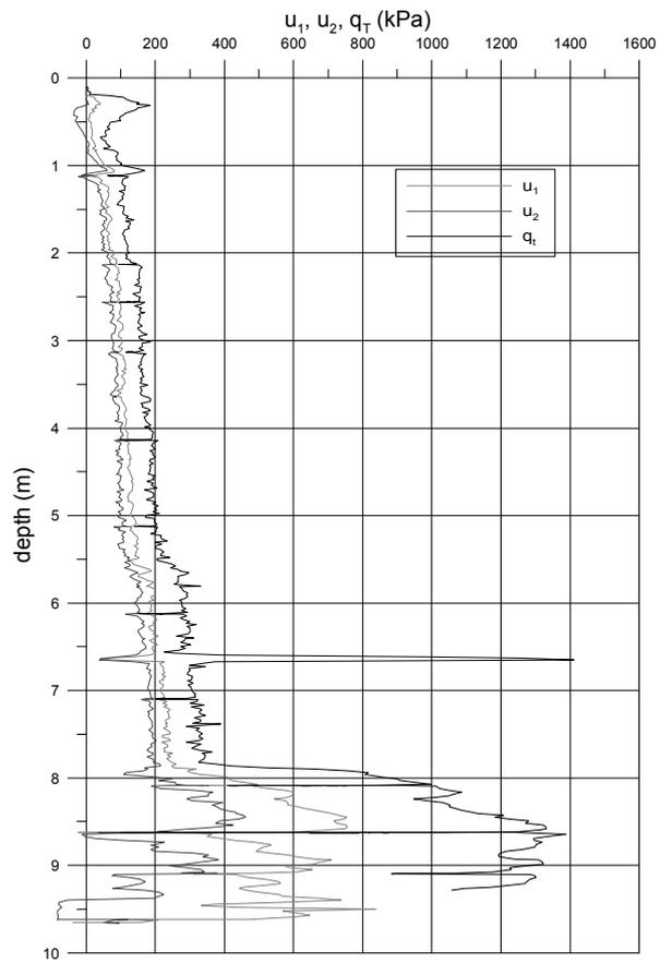
Fig. 4. Typical results of cone resistance ( $q_t$ ) and pore pressure at cone face ( $u_1$ ) and cone shoulder ( $u_2$ ) vs. depth, Sarapuí II soft clay test site (Jannuzzi,2009).
