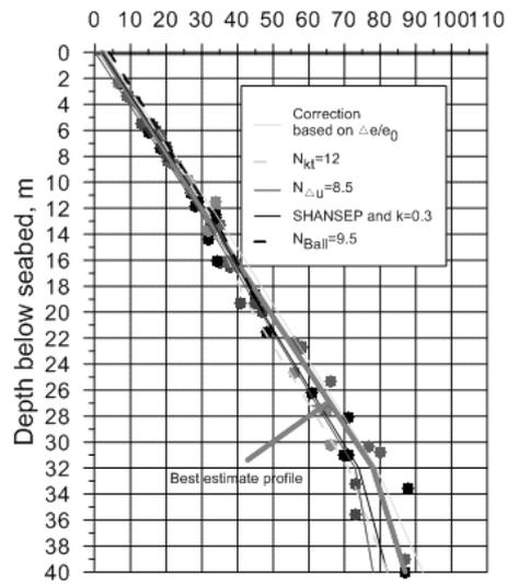
Fig. 16. Undrained shear strength from the four methods
