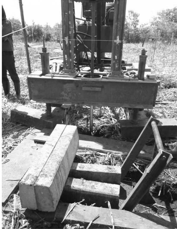
Figure 16 – Detail of the hammer with weight on its top, during a SDMT test.
