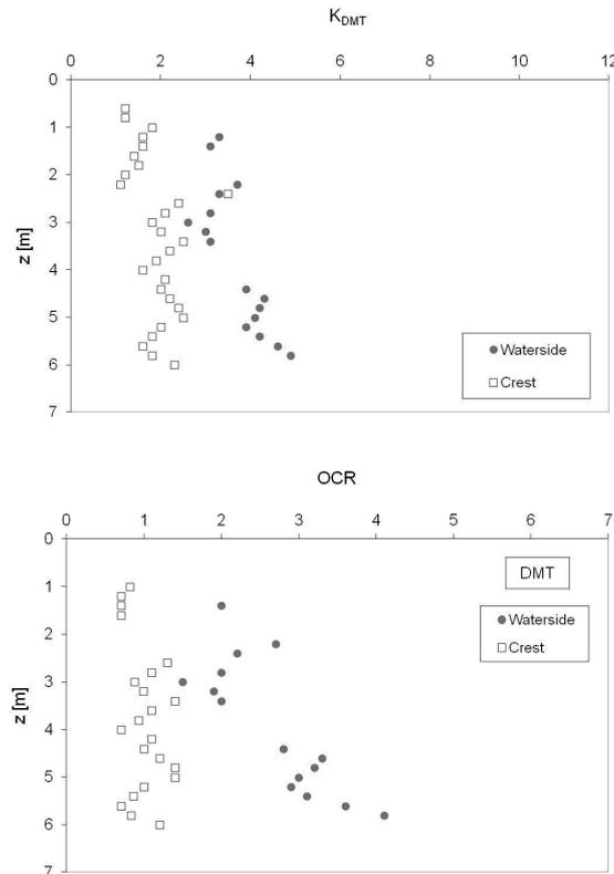
Fig. 4. Lateral stress index  $K_{DMT}$  and overconsolidation ratio  $OCR$  of the dike subsoil
