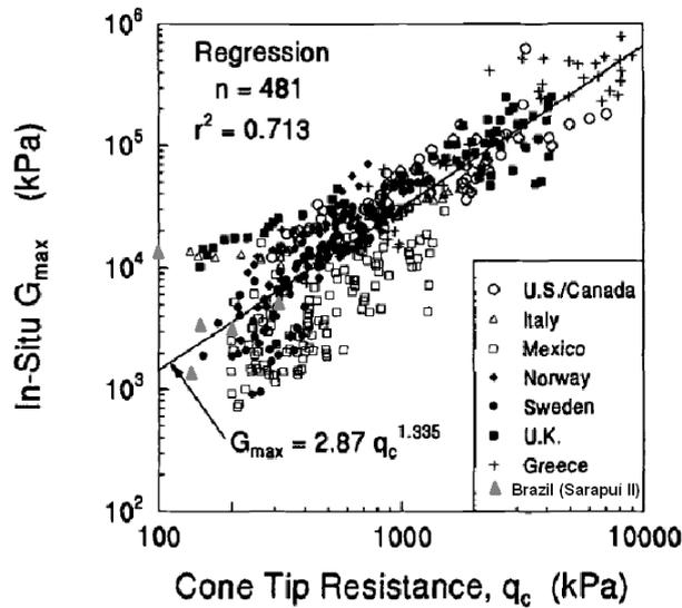
Fig. 22. Apparent relation between maximum shear modulus ( $G_{max}$ ) from in-situ measurements and cone resistance ( $q_c$ ) for clays located worldwide (modified after Mayne and Rix, 1993).
