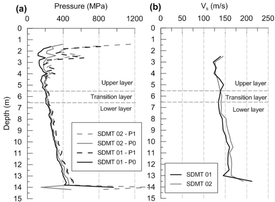
Fig. 5. SDMT test results – measured parameters (a)  $p_0$  and  $p_1$  and (b)  $V_s$
