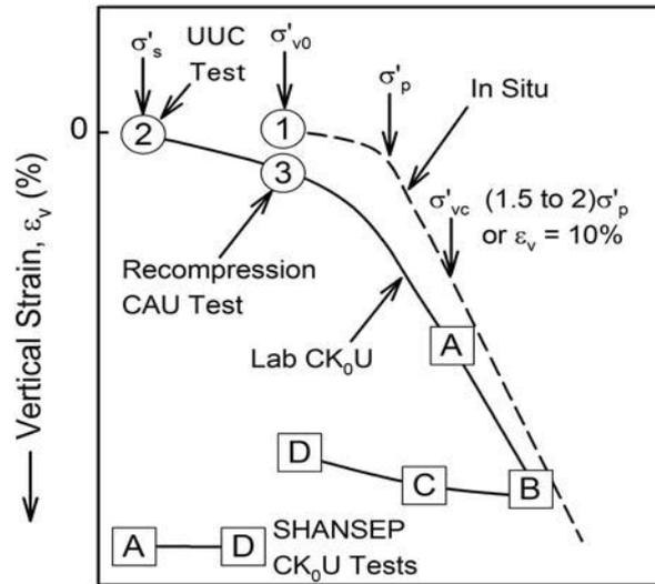
Fig. 1. Recompression and SHANSEP consolidation procedure for laboratory  $CK_0U$  testing (slightly modified from Ladd 1991)
