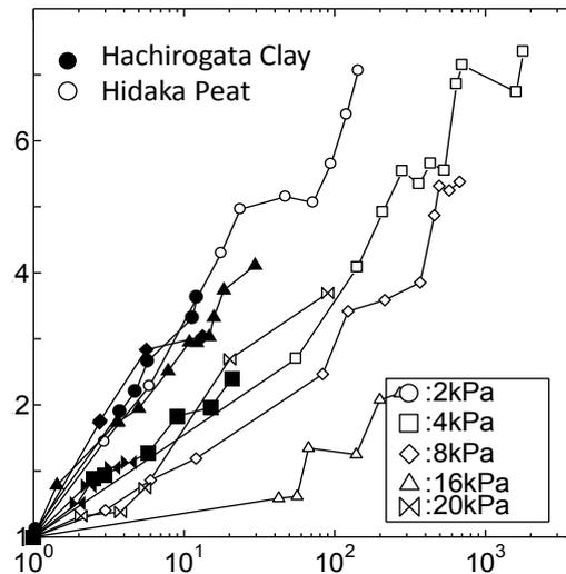
Fig. 7 Increase in  $G$  during secondary consolidation
