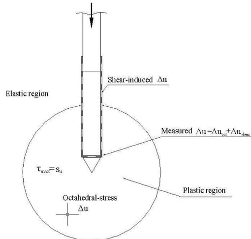
Fig. 7. Soil zones around CPTU probe (after Mayne, 2001)
