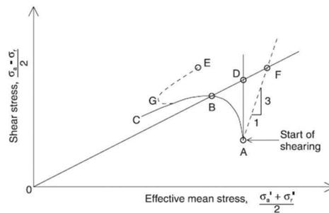
Fig. 7. Correction principle for normally to consolidated to lightly overconsolidated clay from Berre et al. (2007), small strain correction
