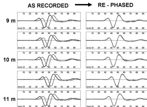
Fig. 2. Example of seismograms obtained by SDMT
