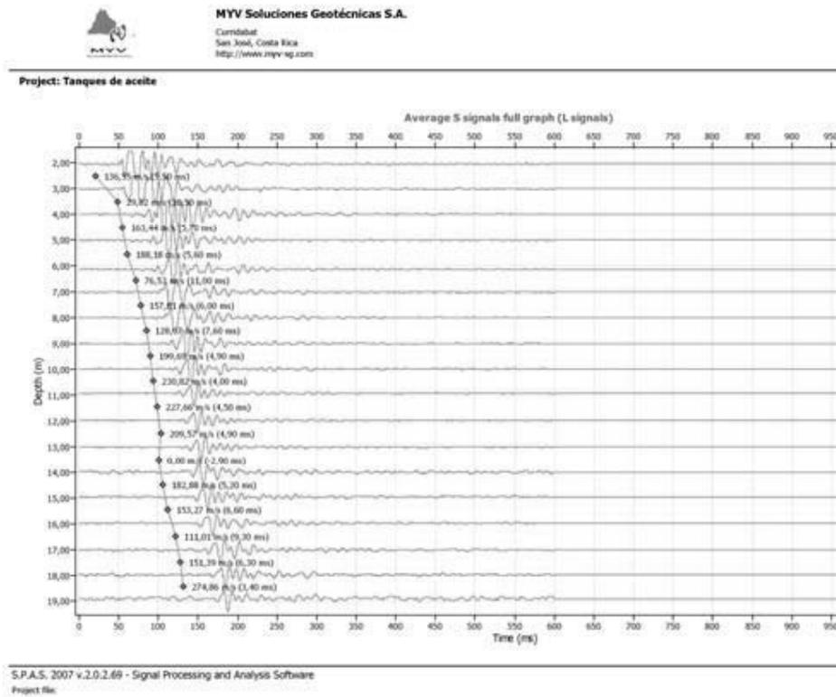
Fig. 15. Data output of the Seismic module.
