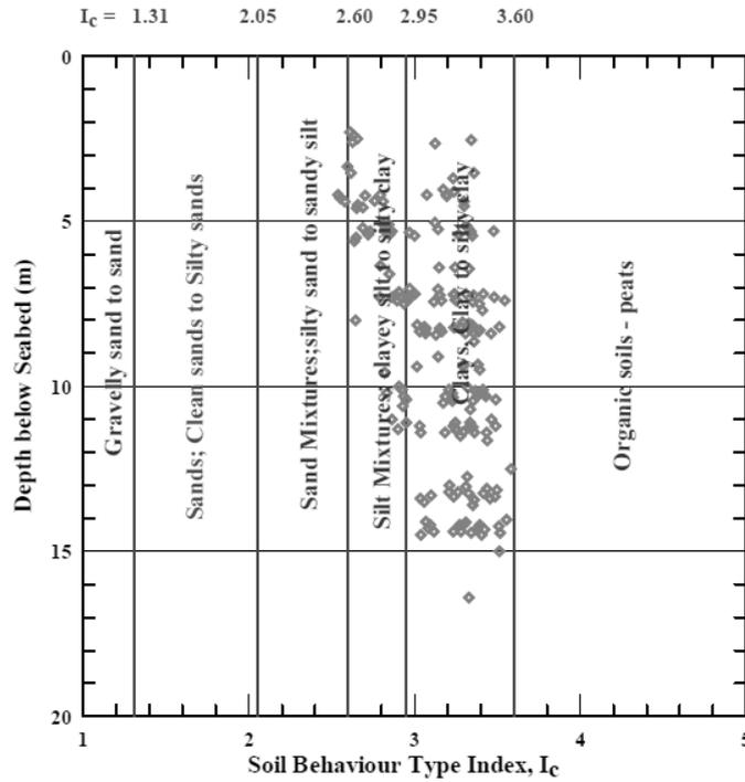
Fig. 1. SBT Index vs. depth
