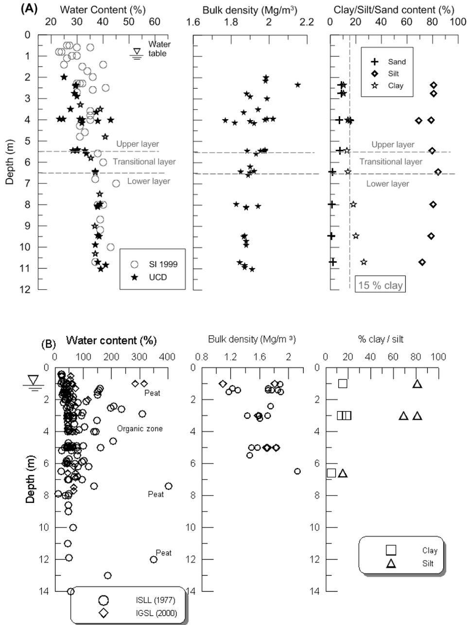
Fig. 2. Stratigraphy and index properties at (a) Foynes and (b) Shannon
