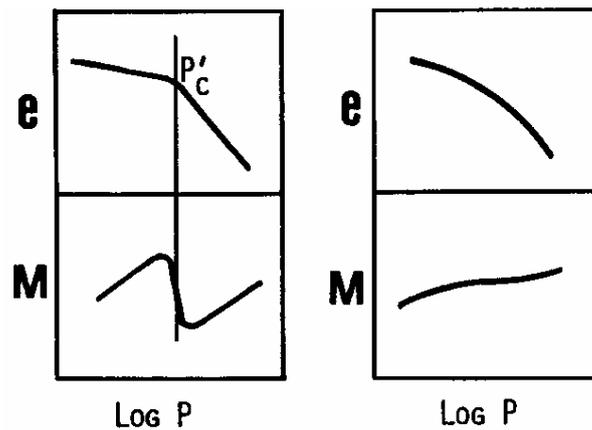
Fig. 1.1 Schematic variation of the oedometer (constrained) moduli with applied load
