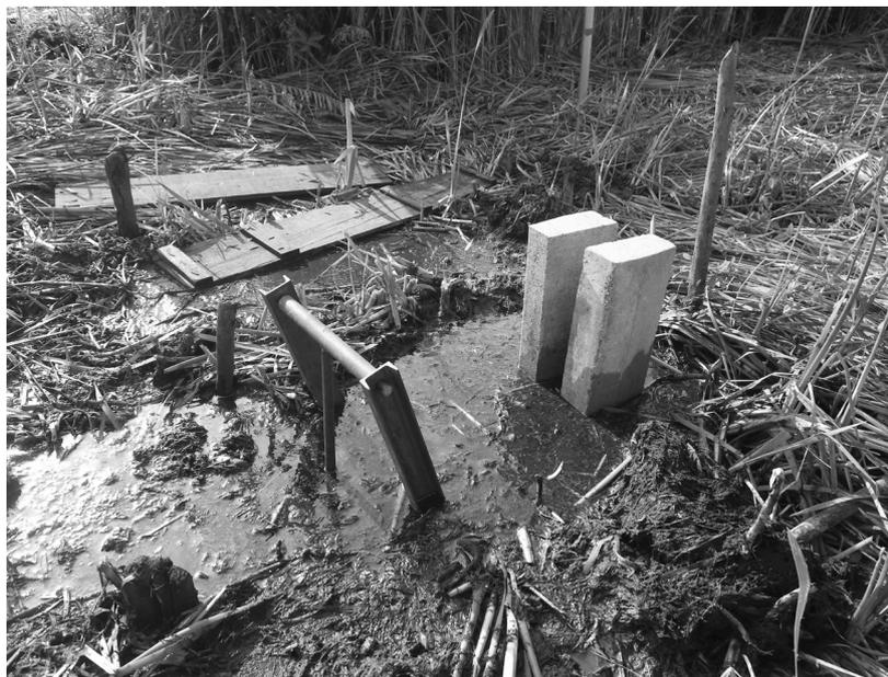
Fig. 9. Hammer in position for the test, with some weight on the top to keep it stable during striking.
