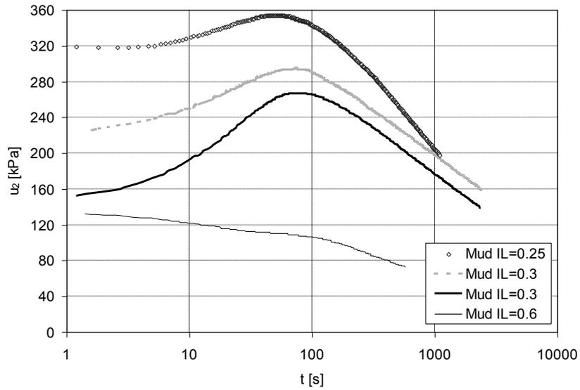
Fig. 11. Set of dissipation curves at the toe of the dike (Bałachowski, 2006b)
