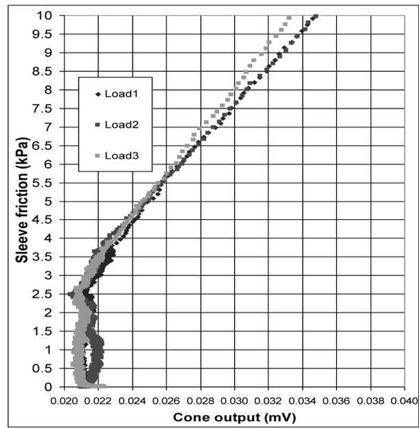
Fig. 6. Influence of dirt seals on sleeve measurements
