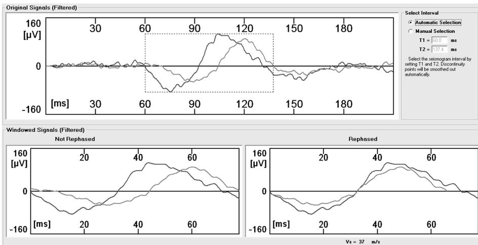
Fig. 18. Seismic dilatometer test performed in the first series of tests, 2.0 m depth.
