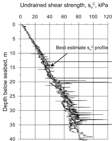
Fig. 12. Undrained shear strength interpreted based on SHANSEP parameters and OCR from CPTU
