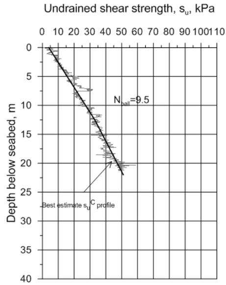
Fig. 15. Undrained shear strength from ball
