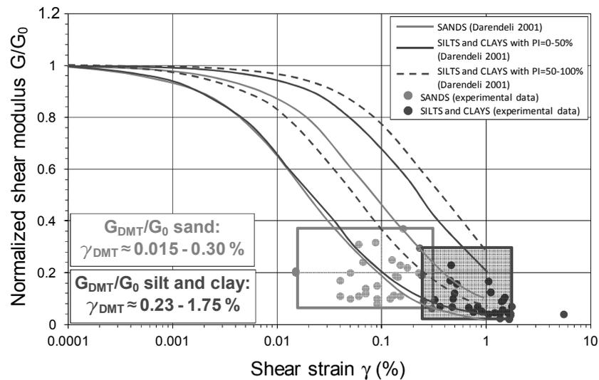
Fig. 9. Use of SDMT data for calibrating the selection of in situ  $G/G_0 - \gamma$  decay curves in various soil types (Amoroso et al. 2014)
