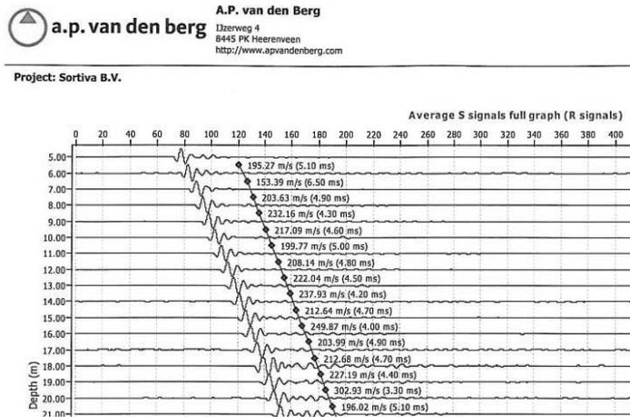
Fig. 5. Results of a series of seismic tests.
