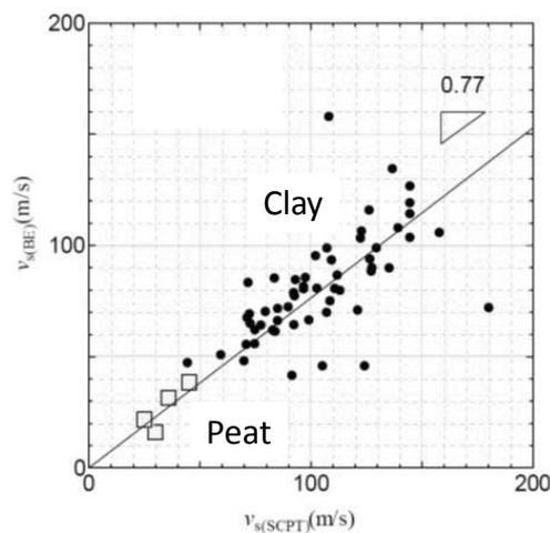
Fig. 6. Sample quality evaluated by shear wave velocity
