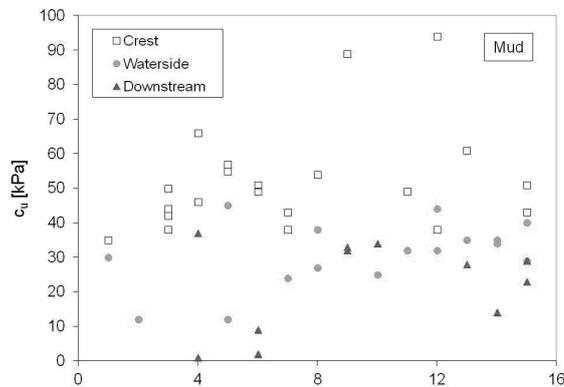
Fig. 6. Undrained shear strength in the mud layers under the dike
