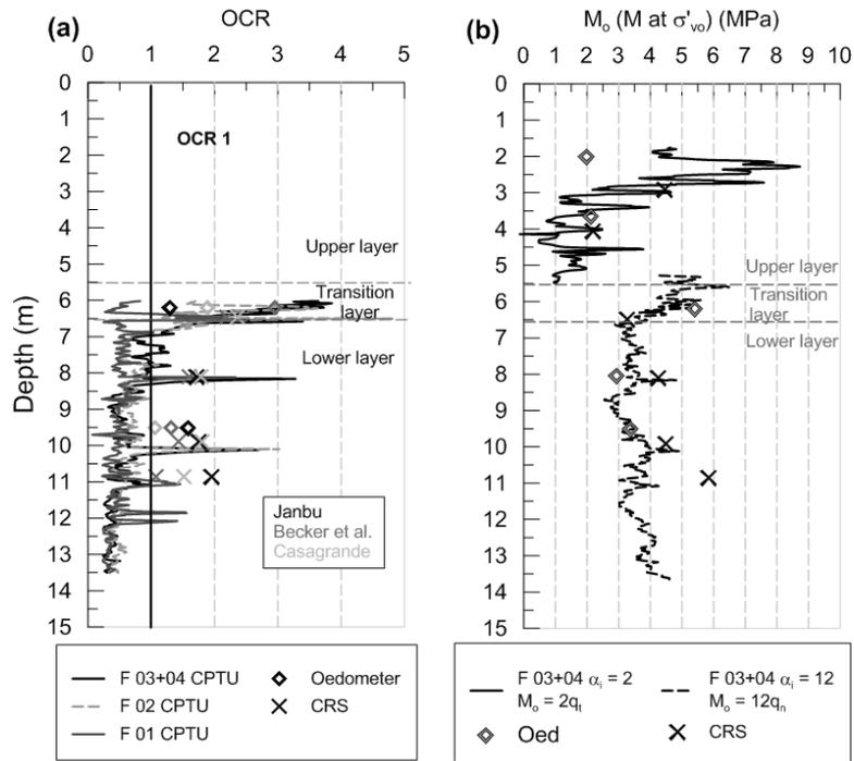
Fig. 12. 1D compression parameters from CPTU for Foynes (a) OCR and (b)  $M_0$ .
