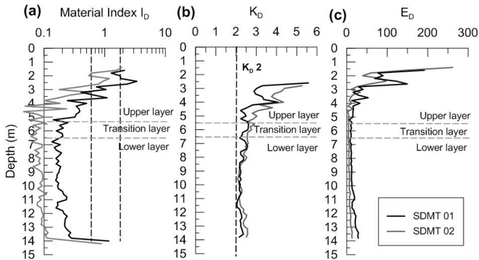
Fig. 6. Secondary SDMT parameters (a)  $I_D$ , (b)  $K_D$  and (c)  $E_D$
