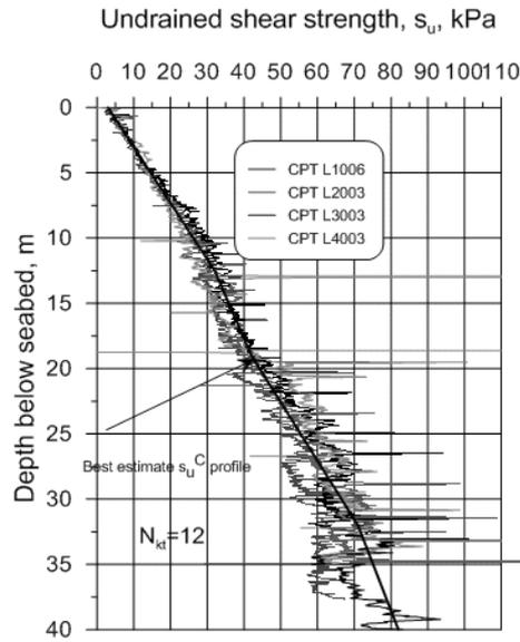
Fig. 13. Undrained shear strength from CPTU,  $N_{kt}$
