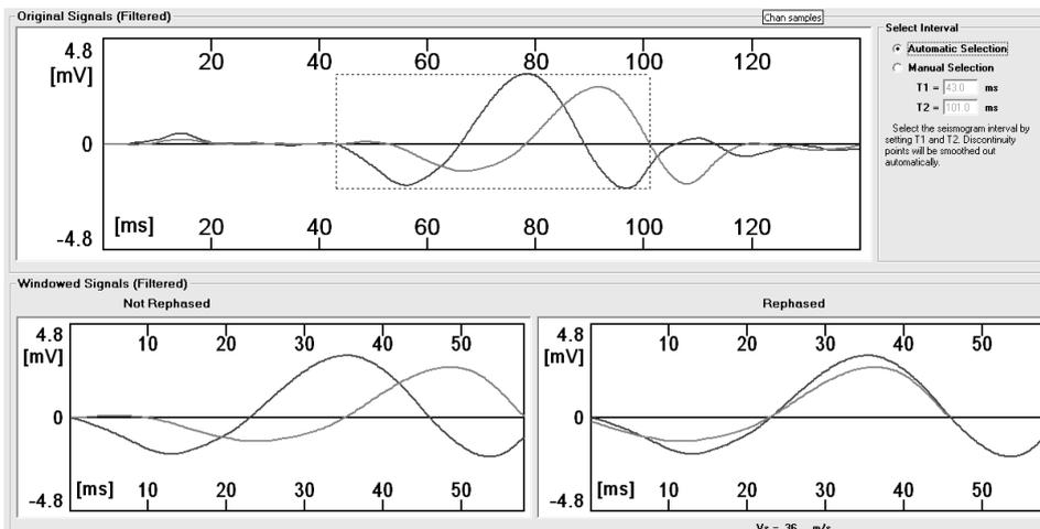
Fig. 19. Seismic dilatometer test performed in the second series of tests, 2.0 m depth.
