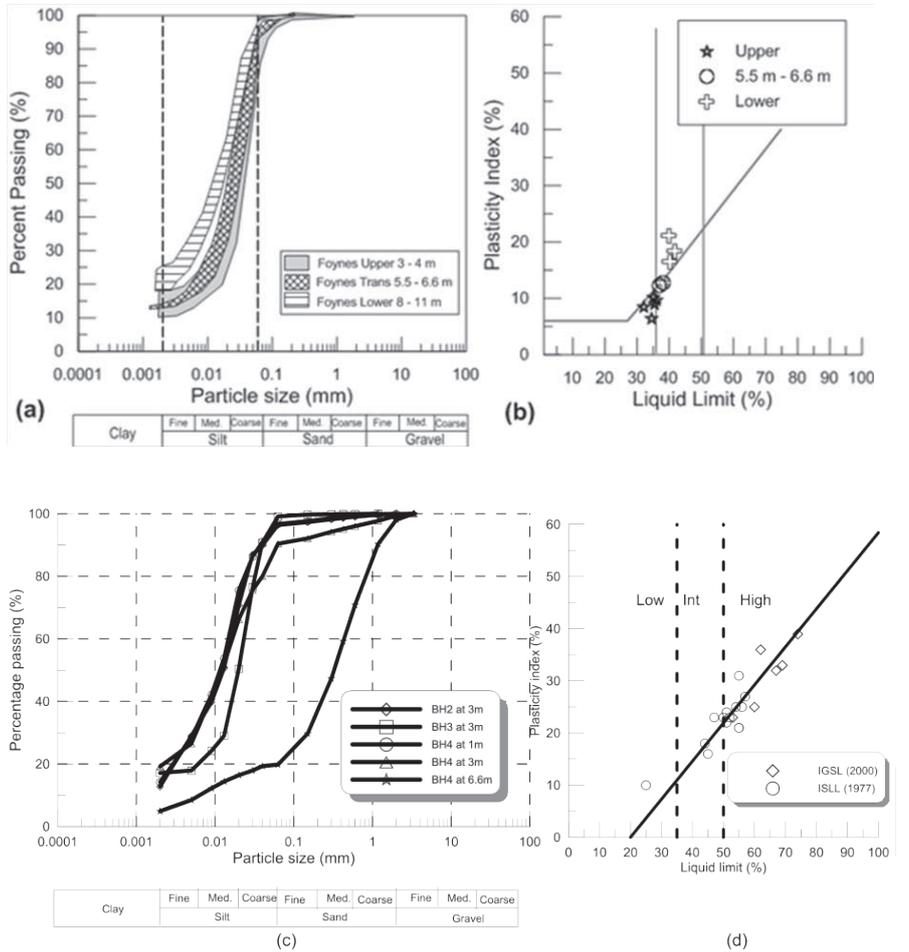
Fig. 3. Results of particle size distribution analyses (a and c) and plasticity chart (b and d) at Foynes and Shannon respectively
