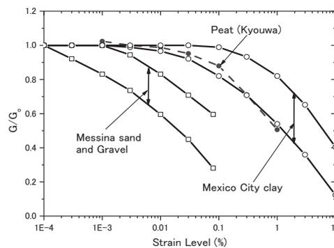
Fig. 9 Strain dependency of small strain stiffness. Lines other than peat are referred from Leroueil and Hight (2003).
