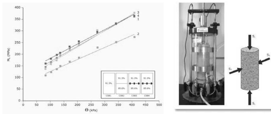
Fig. 4. Resilient Modulus ( $M_R$ ) enhancement from AASHTO T 307
