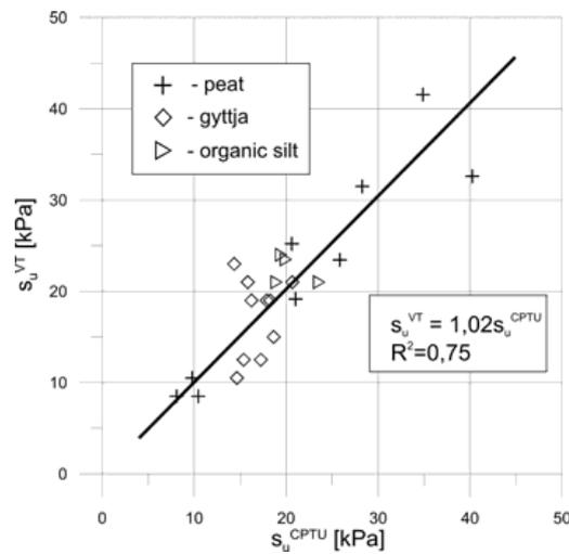
Fig. 12. Comparison of undrained shear values derived from vane test  $s_u^{VT}$  and from piezocone test  $s_u^{CPTU}$ , calculated on the basis of  $N_{kt}$  values given in Fig. 11.
