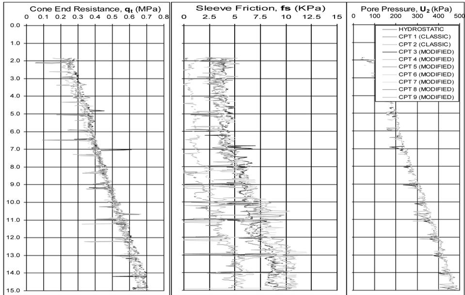
Fig. 13. Test results at Onsøy
