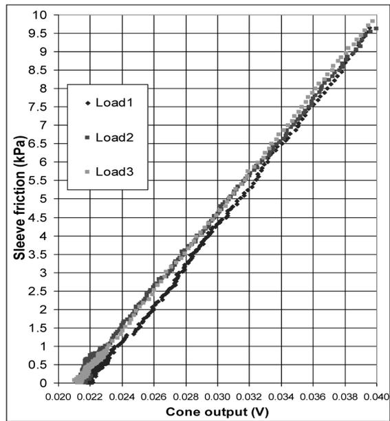
Fig. 9. Sleeve measurements with new spring assembly
