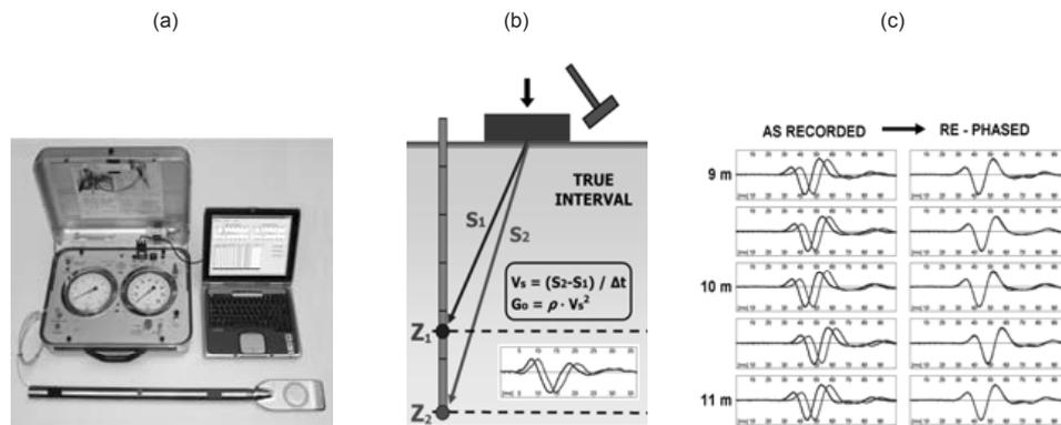
Fig. 2 Seismic Dilatometer: (a) DMT blade and seismic module (b) Schematic layout of the seismic dilatometer test. (c) Example of seismograms as recorded and rephased.
