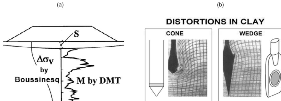
Fig. 4 (a) Settlement prediction by DMT (b) Soil distortions caused by tips of different shape (Baligh & Scott 1975).
