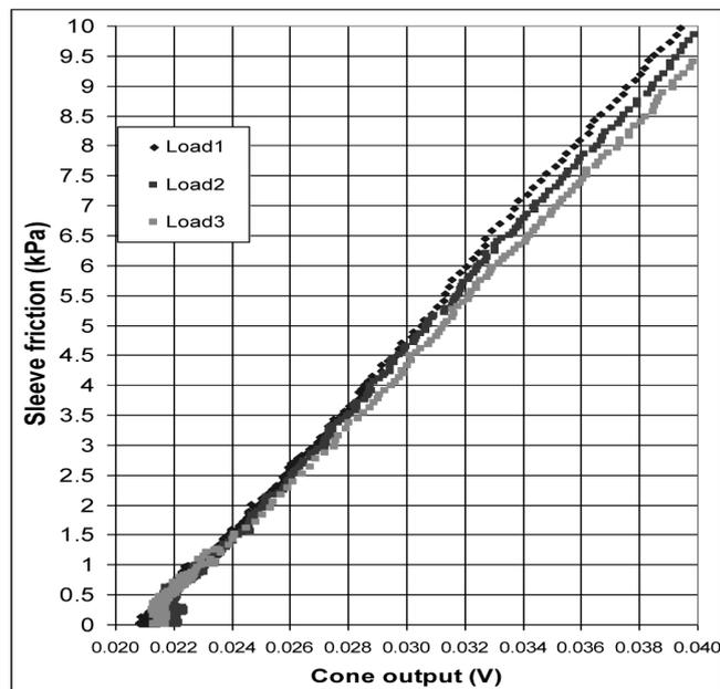
Fig. 5. Influence of O-rings on sleeve measurements
