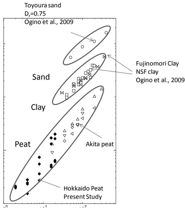
Fig. 8 Relationships between  $G$  and  $p$  for various soil materials
