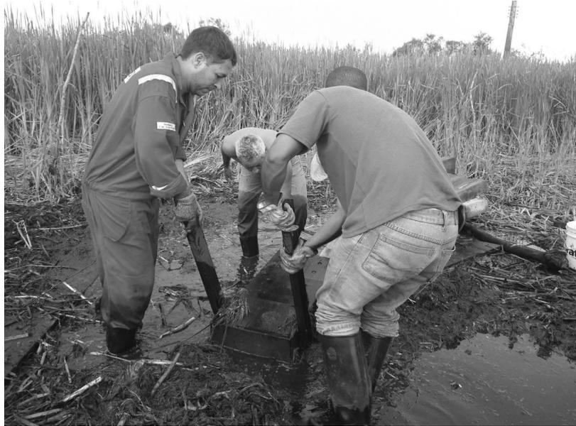
Fig.8. Placement of the hammer on the soil surface, under water.
