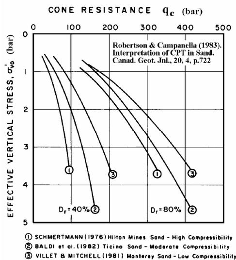
Fig. 6.1 Example of different curves for interpreting  $D_r$  from  $q_c$ .
