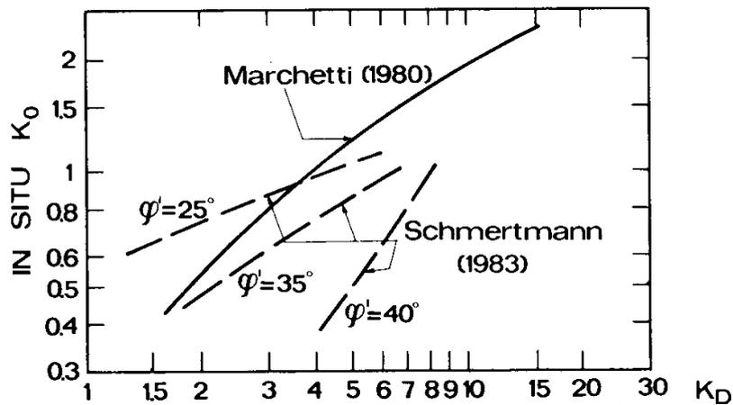
Fig. 4.1 Correlations  $K_o$  vs  $K_D$  as a function of  $\phi$
