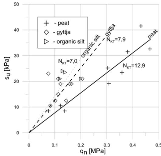
Fig. 11. Linear relationship between undrained shear strength  $s_u$  from VT and net cone resistance  $q_n$ , representing the  $N_{kt}$  values for different soil types
