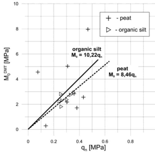
Fig. 9. Correlation between constrained moduli  $M_0$  from DMT and  $q_n$  value from CPTU
