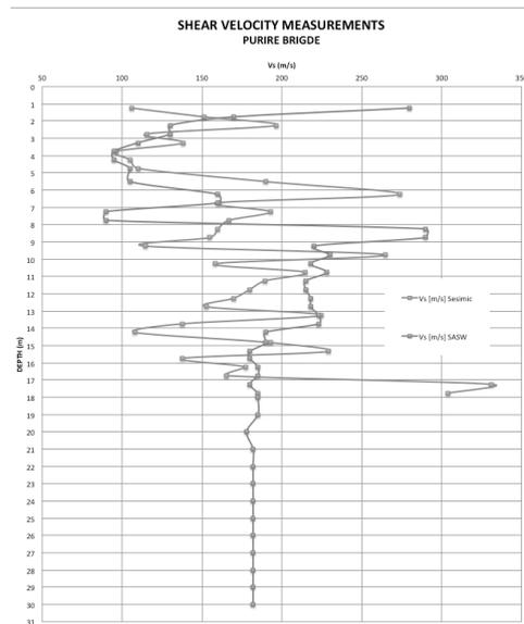
Fig. 13. Comparison between  $V_s$  from SCPTu and  $V_s$  from SASW.
