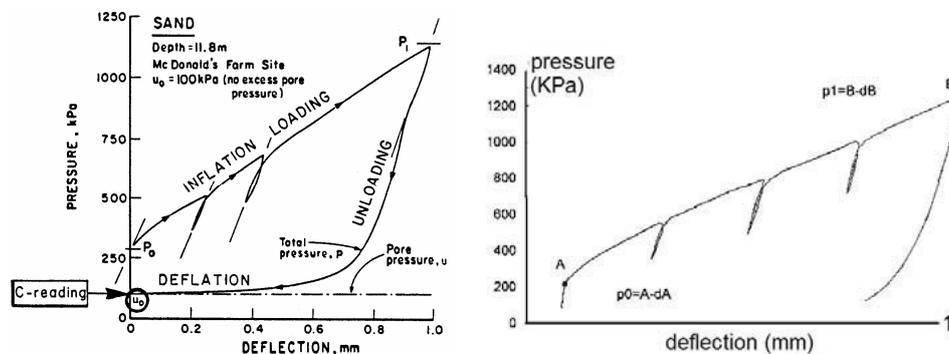
Fig. 5.1 Examples showing the linearity of the pressure-deflection dilatometer curve during inflation. (a) Campanella et al. 1985 (b) Fretti et al. 1992
