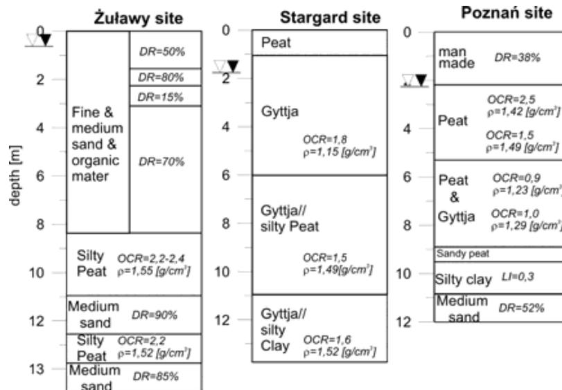
Fig. 2. Geotechnical profiles of the test sites.
