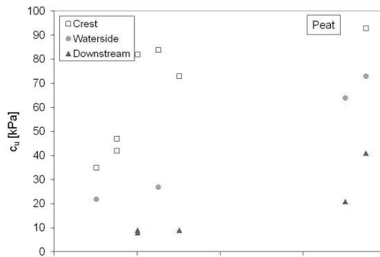
Fig. 5. Undrained shear strength in the peat layers under the dike
