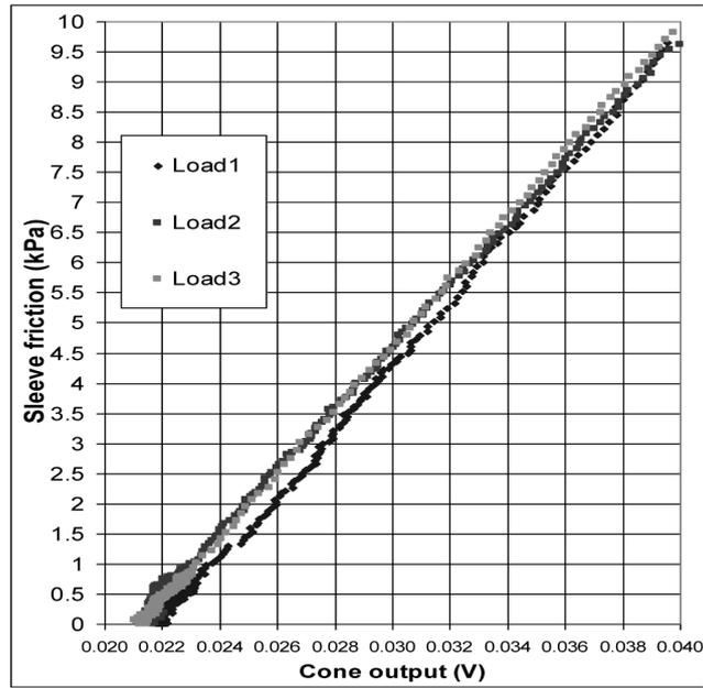
Fig. 4. Sleeve calibration with no seals mounted
