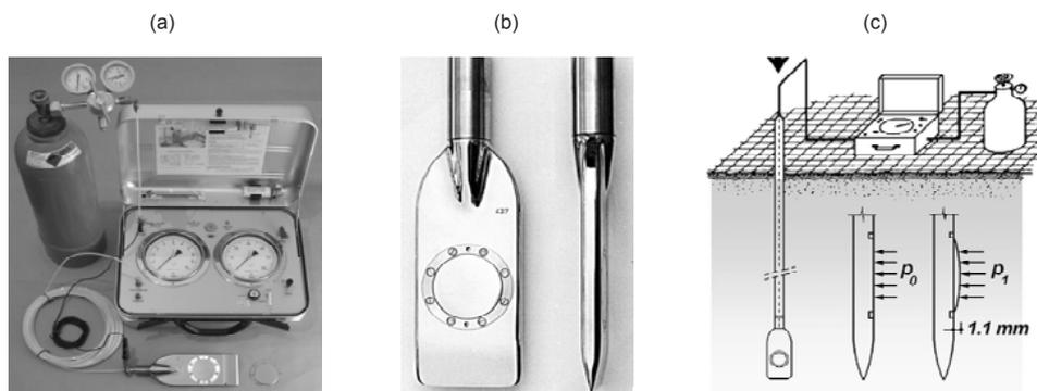
Fig. 1 Flat Dilatometer: (a) Equipment (b) Dilatometer Blade (c) Schematic layout of the seismic dilatometer test.
