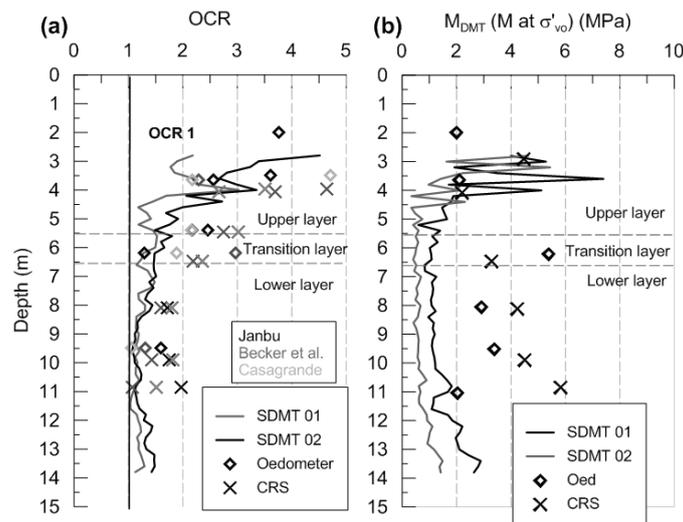
Fig. 11. 1D compression parameters from SDMT for Foynes (a) OCR and (b)  $M_0$ .
