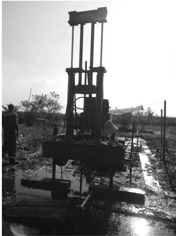
Fig. 6. Rig during SDMT test in Sarapuí II clay.
