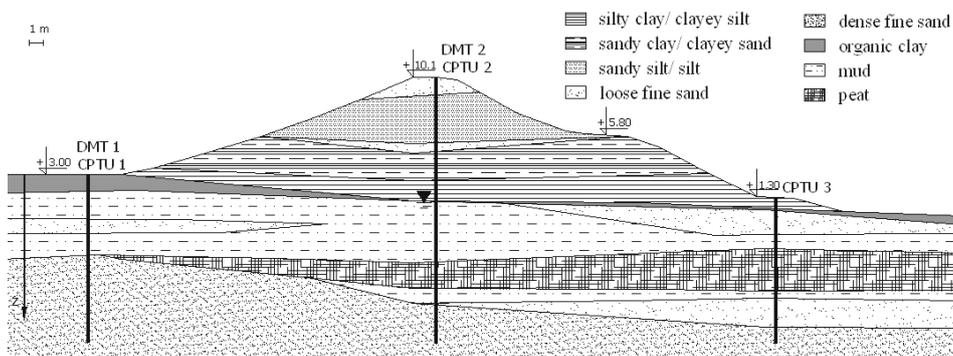
Fig. 1. The dike and its geotechnical cross-section (Bałachowski, 2006b)
