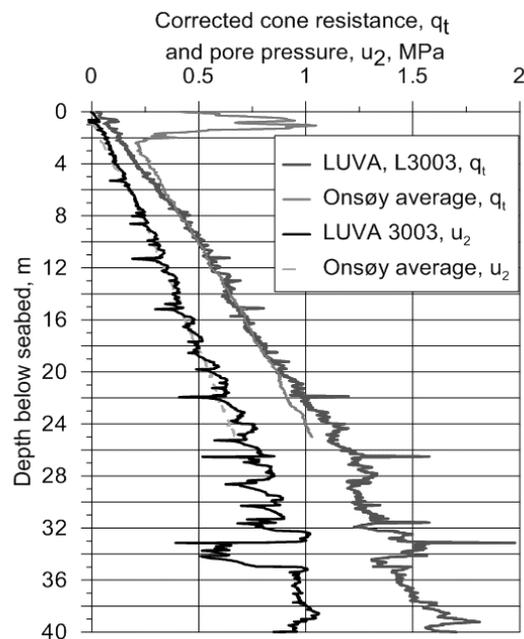
Fig. 5. Corrected cone resistance and pore pressure at LUVA and Onsøy areas
