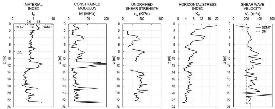
Fig. 4. SDMT results at the site of Cese di Preturo (C.A.S.E. Project), L'Aquila. *On the right*: Comparison of profiles of  $V_s$  from SDMT and Down-Hole (Polo Geologico, MS–AQ Working Group 2010).
