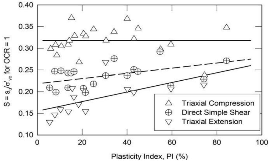
Fig. 2. Undrained strength anisotropy from SHANSEP CK<sub>0</sub>U tests on NC clays and silts (from Ladd 1991).
