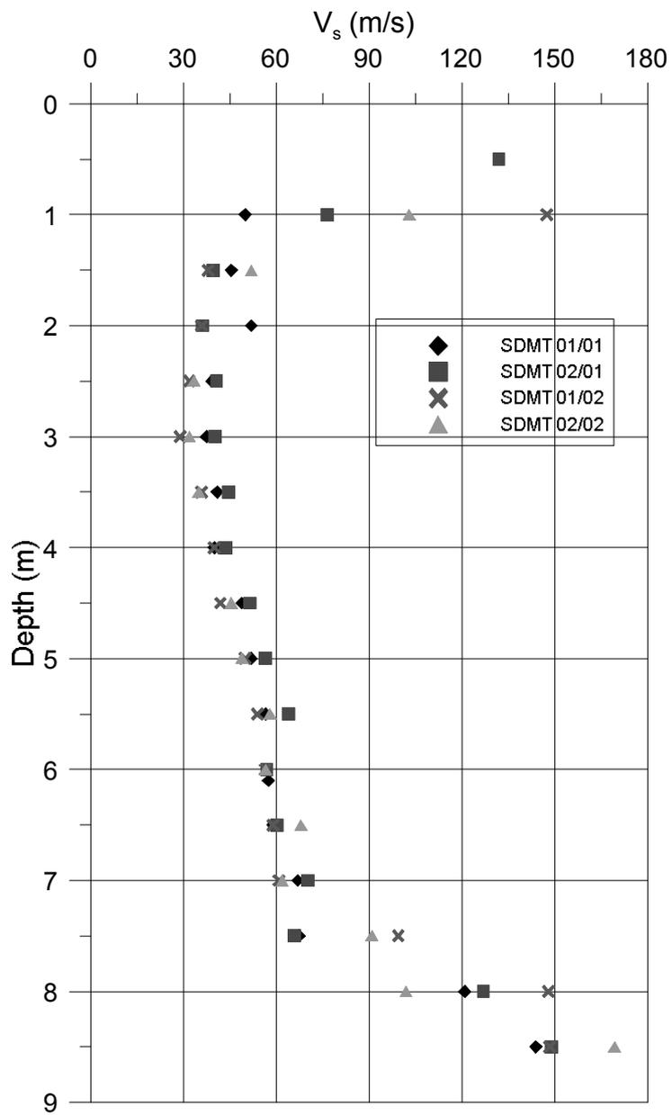
Fig. 20.  $v_s$  values from two series of SDMT tests.
