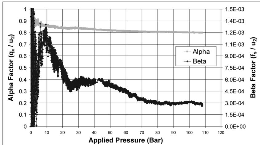
Fig. 3. Calibration of Beta factor (Beta vs chamber pressure)
