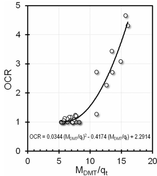
Fig. 4.4 Correlation  $OCR = f(M_{DMT}/q_c)$  for the Venice Lagoon Sandy layers (Monaco et al. 2014)
