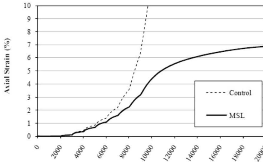
Fig. 7. Repeated load deformation tests for unbound control aggregate and mechanically stabilized layer incorporating one of TriAx geogrid (Wayne 2010)
