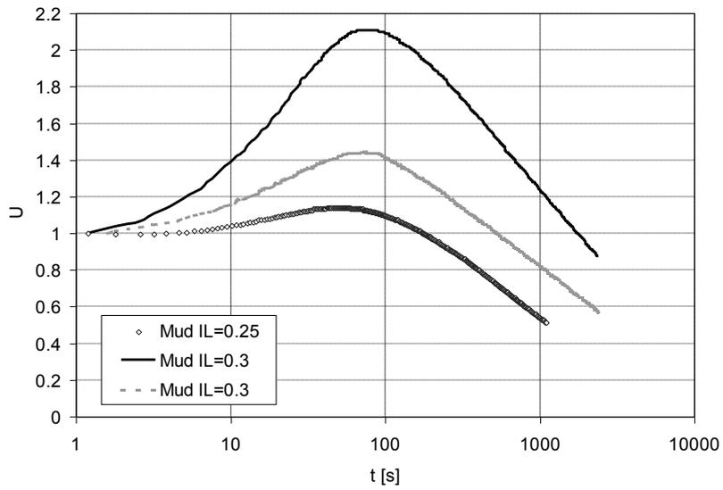
Fig. 12. Set of normalized excess pore water pressures at the toe of the dike (Bałachowski, 2006b)
