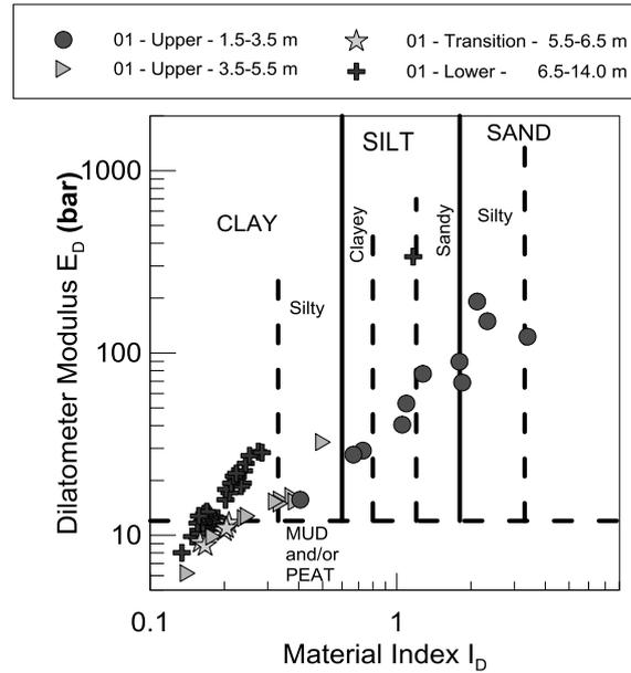
Fig. 9. Foynes SDMT data plotted on chart of Marchetti and Crapps (1981)
