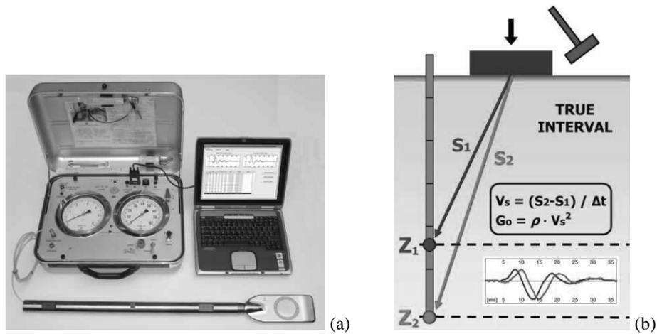
Fig. 1. Seismic dilatometer test. (a) DMT blade and seismic module. (b) Schematic test layout.
