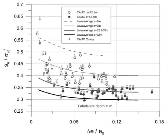
Fig. 9. Normalized compression shear strength as function of  $\Delta e/e_0$
