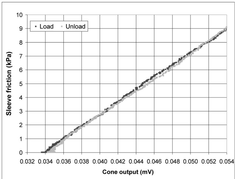
Fig.11. Load – Unload with new spring assembly
