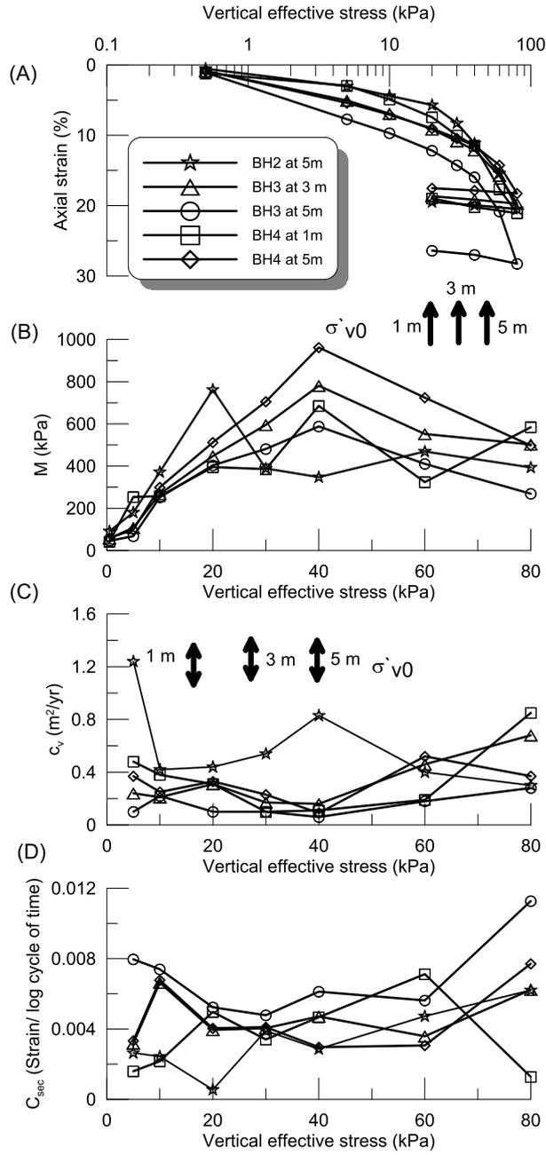
Fig. 10. Oedometer tests for Shannon presented in (a) conventional  $\log \sigma'_v$  versus  $\epsilon$  format (b)  $M$  versus  $\sigma'_v$ , (c)  $c_v$  versus  $\sigma'_v$  and (d)  $C_{sec}$  versus  $\sigma'_v$
