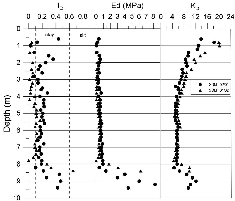
Fig. 17.  $I_D$ ,  $E_D$  and  $K_D$  versus depth.
