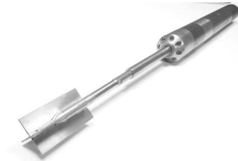
Fig. 10. Icone vane (without protection tube).
