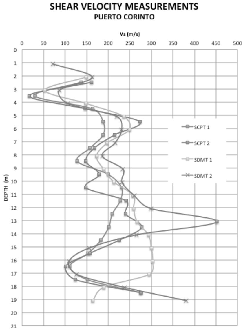
Fig. 16. Comparison of the shear velocity between two different sets of equipment.
