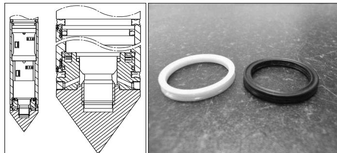
Fig. 1. Influences on the friction sleeve (left) drawing courtesy of AP Van Den Berg. Dirt seals: plastic 'V' shaped lip-seals and rubber quad-o-rings (right)
