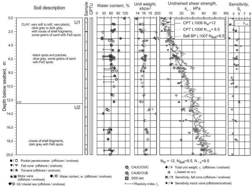
Fig. 2. Soil profile between 0-20 m for one borehole at the LUVA location
